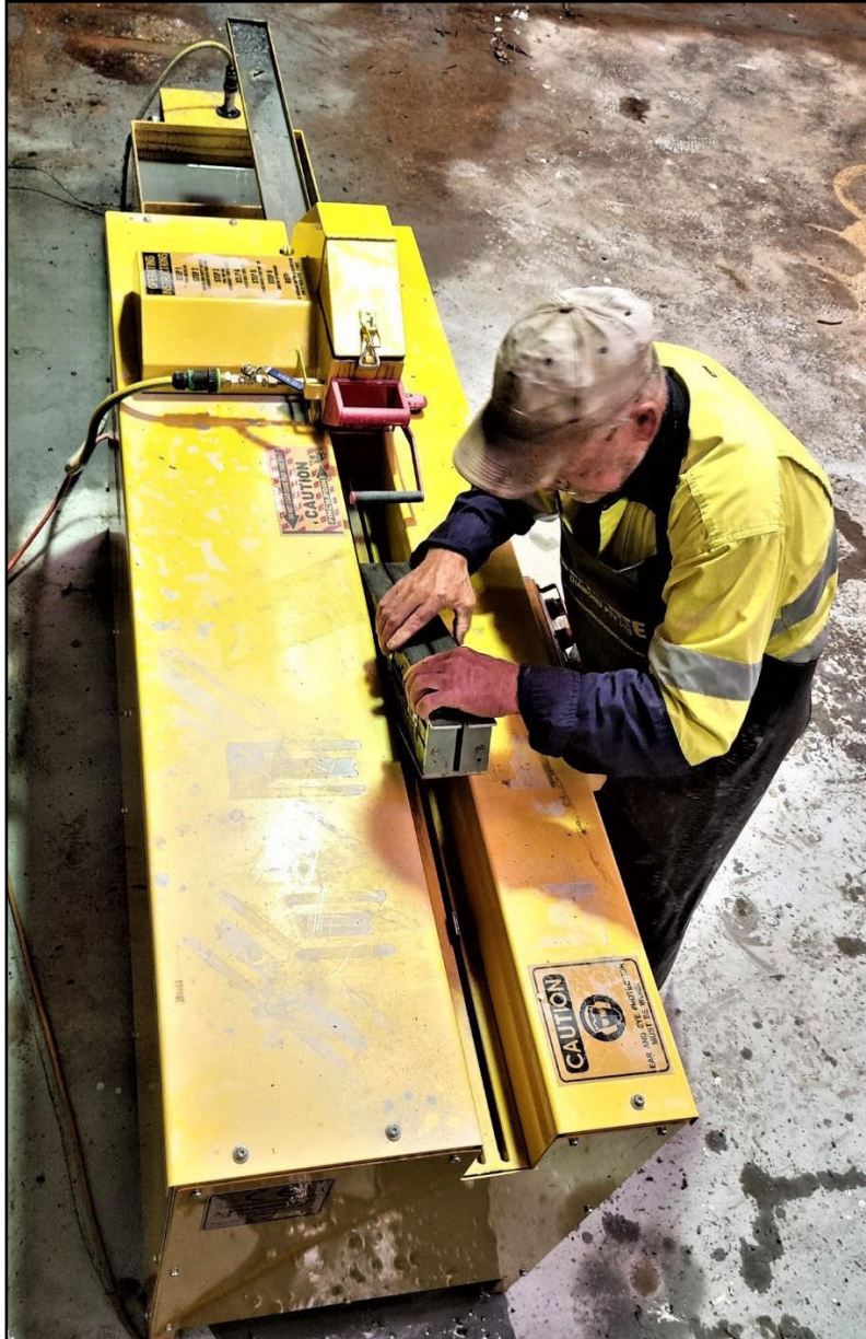
Photo 1 Almonte Auto Core Saw in Nagambie's Core Shed
