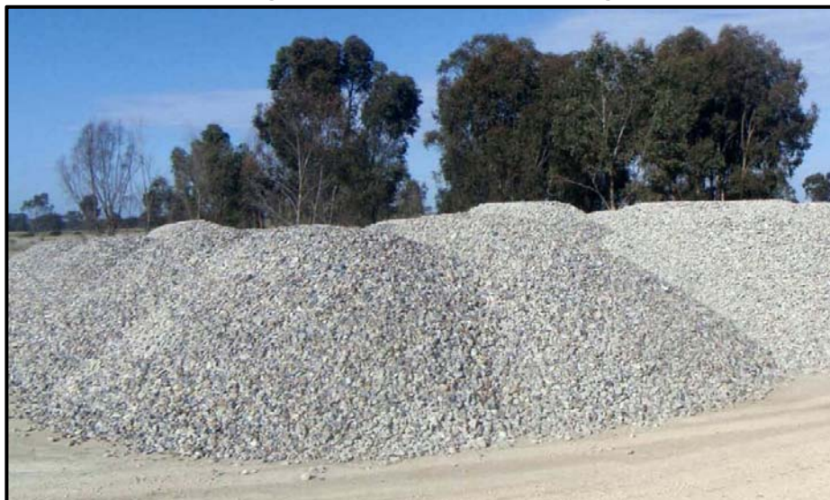
Photo 2 40mm minus gravel on the sales pad at the Nagambie Mine
