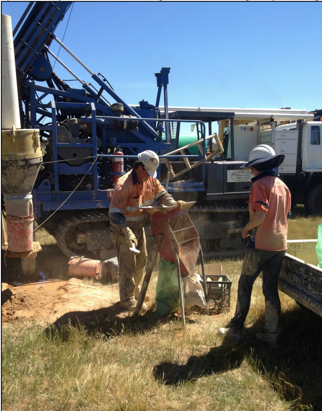
Split for assay collected in calico bag with remainder in green plastic bag
