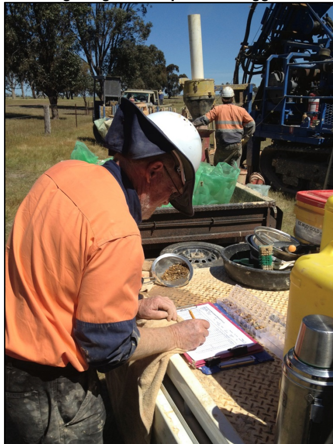
Typical rock chips are retained in a plastic tray and the geological interpretation logged
