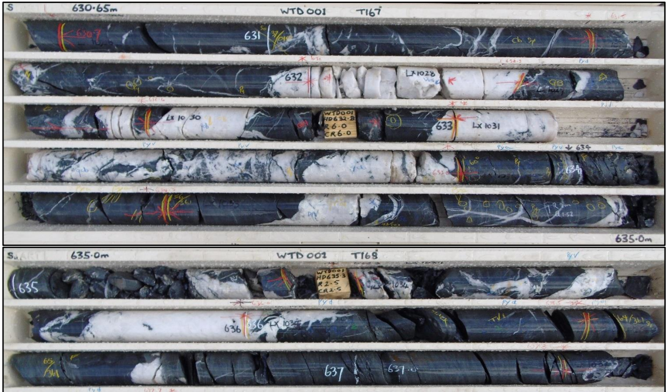
Photo 1 WTD001 intersection of Wandean Thrust Fault zone from 631.5m to 636.5m downhole
