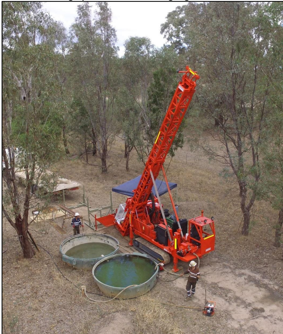
Photo 1 Setting Up the Diamond Drilling Rig for Hole NAD001
