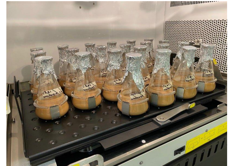
Stage 1: Shake flasks used for bioleaching experiment.
