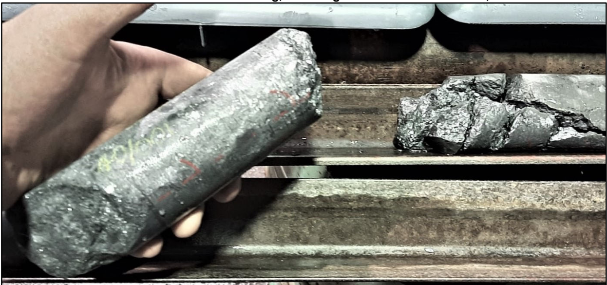
Photo 2 Some of the Massive Stibnite Veining, including Solid near-100% Stibnite, in NAD009
