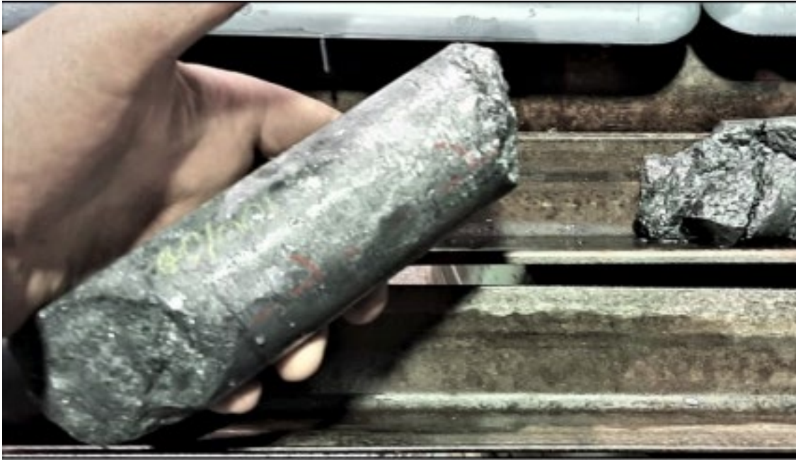
Massive Stibnite Veining in NAD009
