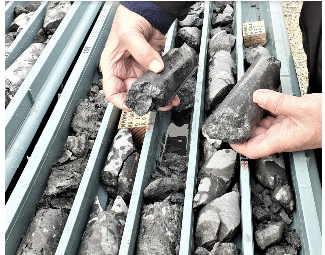
Massive Stibnite Veining in NAD009 and NAD010
