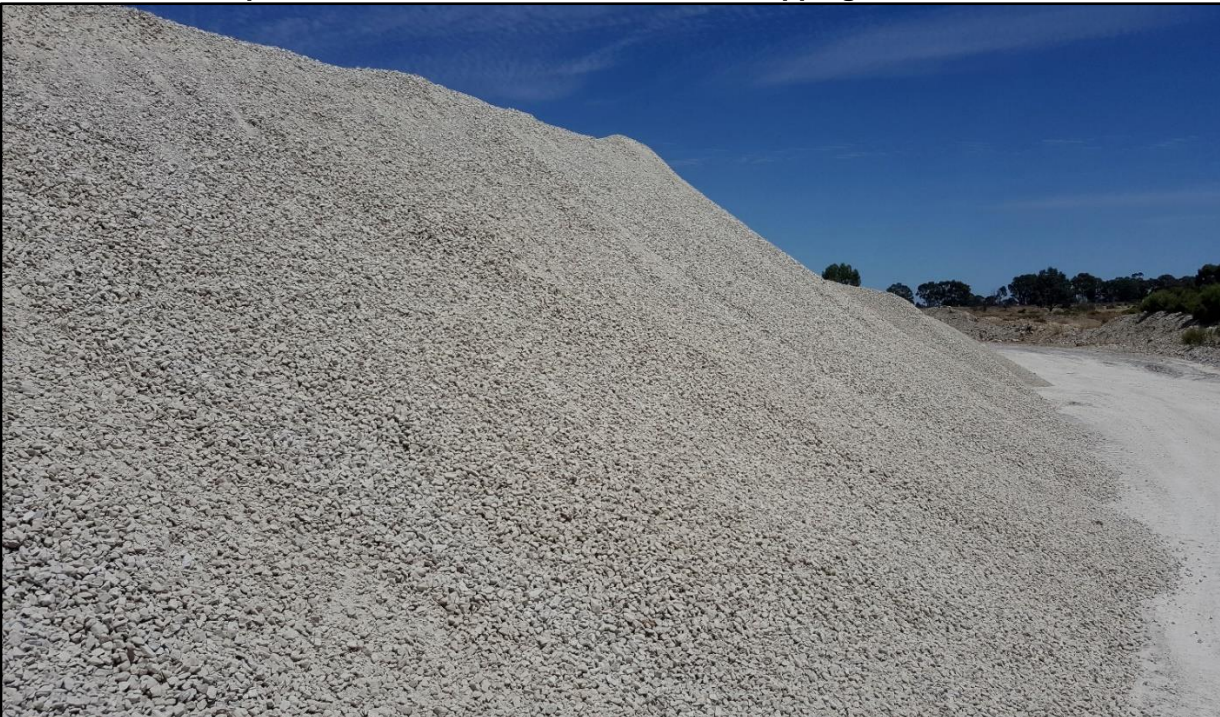
Photo 5 Close-Up View of 20 mm minus Class 4 Road Topping Gravel
