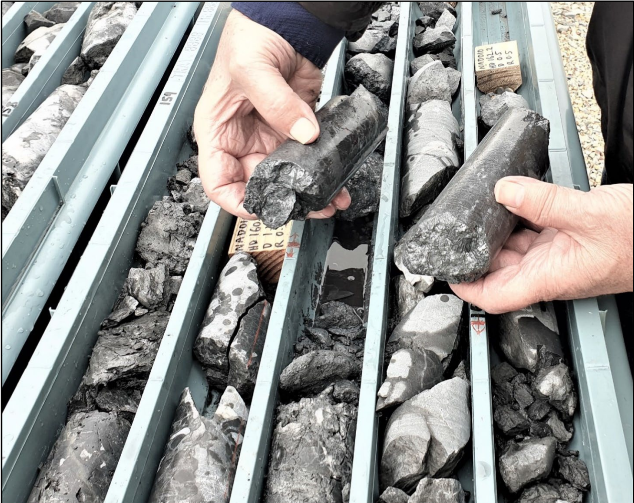
Photo 3 Some of the Massive Stibnite Veining in NAD010**
