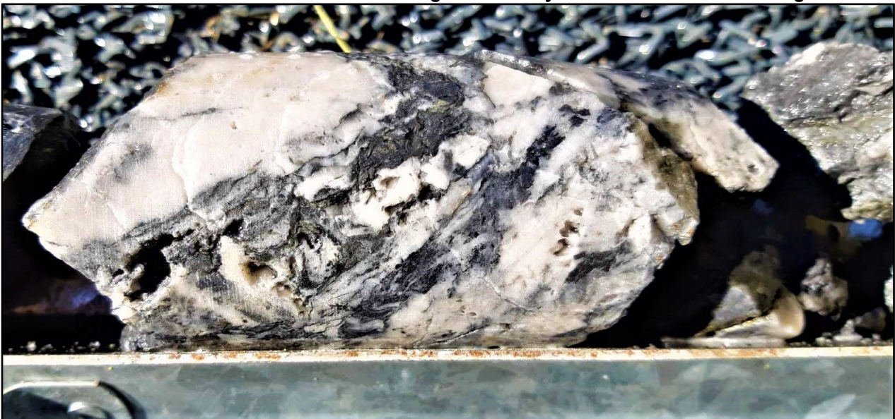
Photo 4 Some of the Laminated Quartz Veining Immediately East of the Stibnite Veining in NAD010
