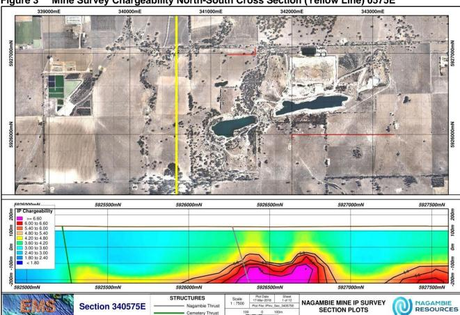
Figure 3 Mine Survey Chargeability North-South Cross Section (Yellow Line) 0575E
