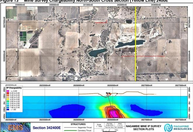
Figure 13 Mine Survey Chargeability North-South Cross Section (Yellow Line) 2400E
