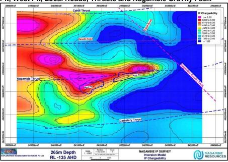
All the IP "hot zones" (red and purple coloured high chargeability contours) for the Nagambie Mine target in the plan and the 12 cross sections are adjacent to the aeromagnetic-interpreted, east-west-striking Nagambie Thrust, conforming with Nagambie Resources' gold deposition model.
