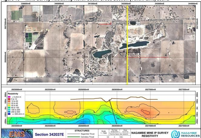
Figure 15 Mine Survey Resistivity North-South Cross Section (Yellow Line) 2037E
