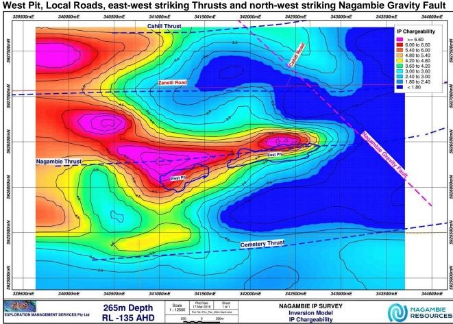
Figure 2 Plan View showing Slice through Mine Survey 3D IP Model at 265m Depth, East Pit, West Pit, Local Roads, east-west striking Thrusts and north-west striking Nagambie Gravity Fau
