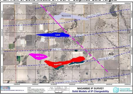
In the 1990s Perseverance Mining mined 180,000 ounces of surface oxide gold from two open pits (refer above figure) on the only outcropping lode at Nagambie, unaware that the other three buried sulphide targets existed. The most intense IP chargeability anomaly, Cahill, is 1.5 km north of the Nagambie Mine and commences only 100m below surface.
