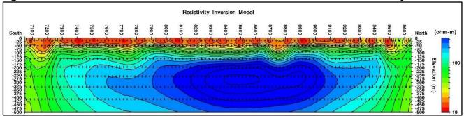
Figure 5 shows the Zonge Inversion-Modelled Resistivity along the same section. The higher chargeability zones coincide with a broad zone of high resistivity.
