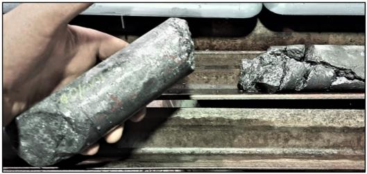
Photo 1 Solid Massive Stibnite Veining in NAD009
