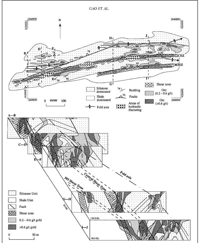
FIG. 3. A. Geologic plan of 120 m RL showing lithology, structure, and gold distribution. Areas of hydraulic fracturing are also shown. B. Cross sections between 130.0 m RL and 90.0 m RL, showing fold, shear zones, and the shape and distribution of the ore blocks.
