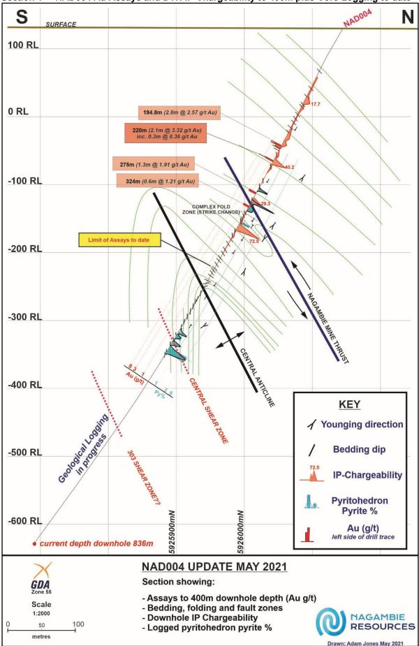
Section 1 NAD004 Au Assays and DTH IP Chargeability to 400m plus Core Logging to date
